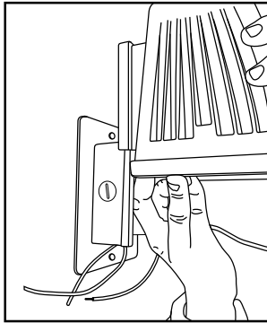
Slide fixture housing onto mounting box
